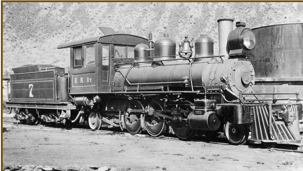
Eureka Nevada Railway Number 7 was one of several new Porter locomotives purchased while John Sexton ran the railroad. The trim little 2-6-2 had nice lines, but was said to be "slippery," and was not well-liked by crew or management. Fred Jukes photo, author's collection.
