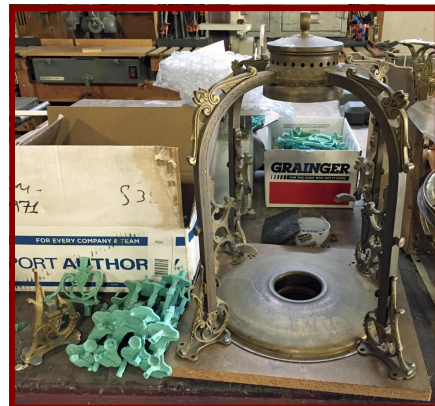
Lamp produced in 1983 by Shortline Enterprises, and the moldings that will be used to make the castings for the new lamps.
