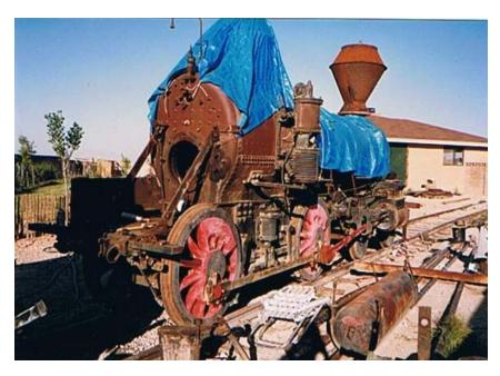
Now that I had all these things apart, it was time to evaluate it all and repair what needed repairing. Many of the items removed would simply have to be replaced, such as the ash pan. Sometime in the early part of the 20th century, the railroad had converted the locomotive from wood to oil. Since I was to rebuild *Eureka* to burn her original fuel of wood, I could see that a wood-burning ash pan and grates needed to be built along with grate bearers.
