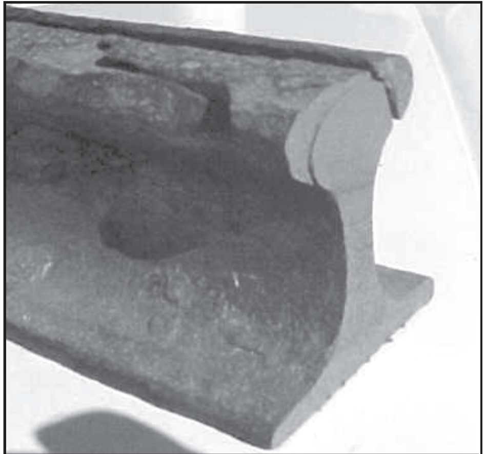
Crystallized rail from the Virginia and Truckee Railroad. Note the lamination and separation. NSRM Collection
